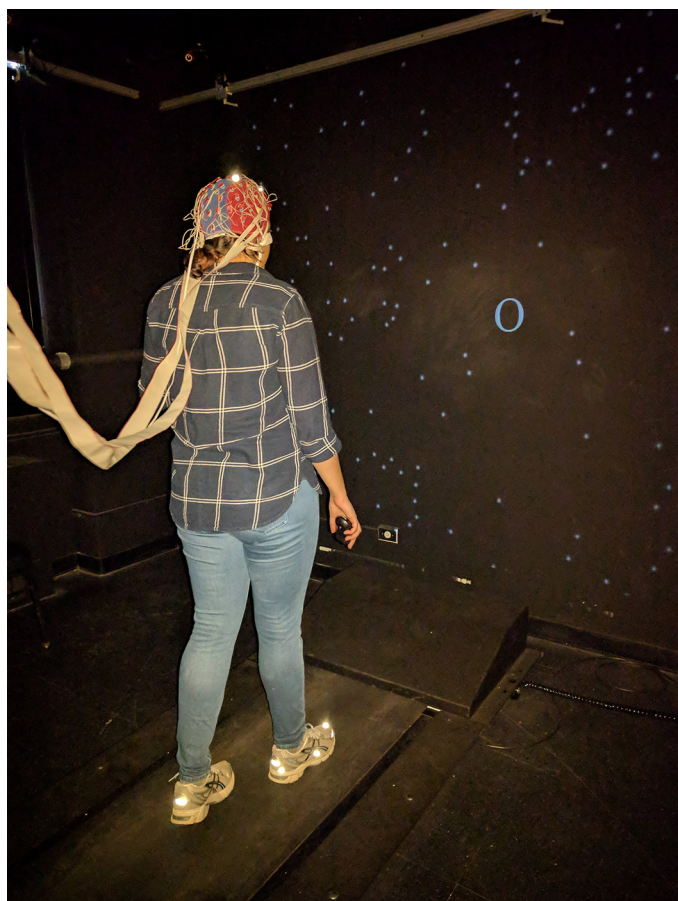
Fig. 1. Representation of recording apparatus. A participant is shown walking on the treadmill facing the optic flow display while wearing a 72-channel EEG cap, with motion capture markers on the head and feet.
