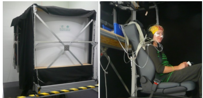
Figure 1. (Left) The outside of the Stewart platform. (Right) A subject with EEG electrodes in place, ready to perform the task. During this study, a cloth sheet covered the platform to mask visual motion cues, and a Biosemi ActiveTwo EEG system was installed to record EEG data.
