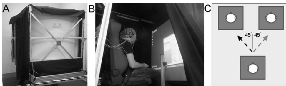
Fig. 1 (Left) The outside of the Stewart platform. (Middle) During this study, a cloth sheet covered the platform to mask visual motion cues, and a Biosemi Active Two EEG system was installed to record EEG data. (Right) Top-down view of the experiment. Example of the
