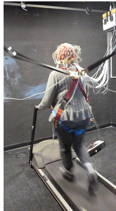
Fig. 1. Illustration of a participant walking on the treadmill wearing an EEG cap and foot pressure force sensors while performing the Go/NoGo-task.
